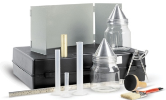
Sand Patch Apparatus
