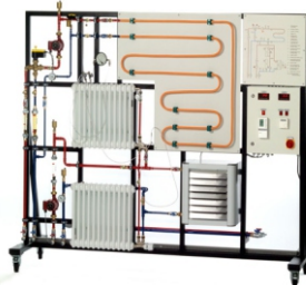
Energy Losses In Pipes
