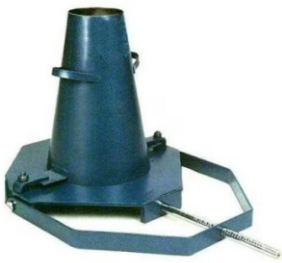
Slump Cone Test Apparatus
