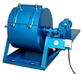
Los Angeles Abrasion Testing Machine
